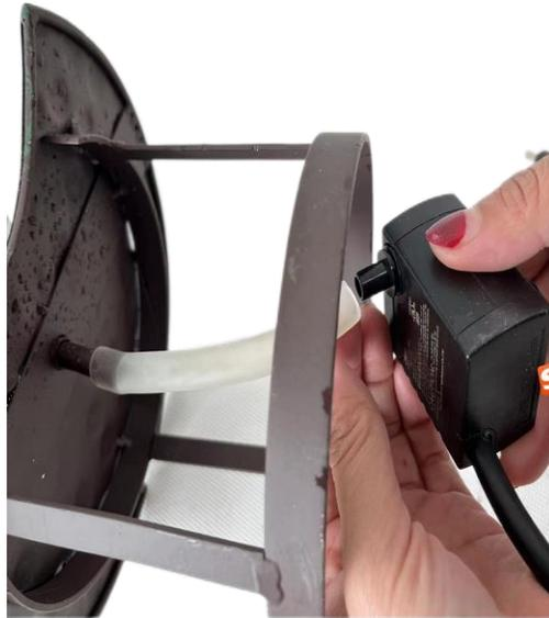
Locate and attach the pre-installed tubing to the output of the pump.
