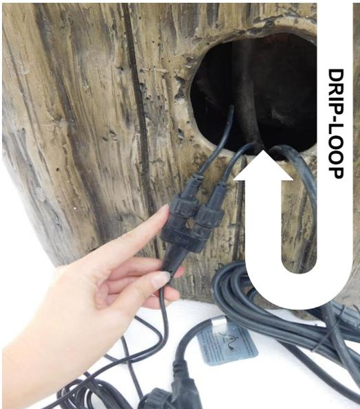
Retrieve the light connector from inside the fountain. **The light connection must sit outside the fountain.** **IMPORTANT:** to prevent water loss during operation, create a drip-loop with the light cords by dipping them into the reservoir before they exit out the back of the fountain.
