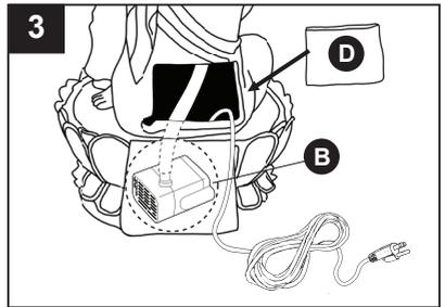
4. Fill the water reservoir with enough water to completely submerge pump (B). Connect the power cord into an electrical socket to run the fountain.
