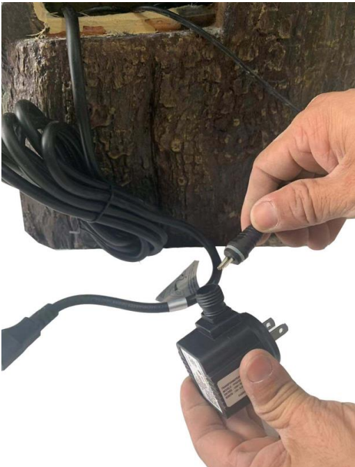
Locate and retrieve the light connection from inside the fountain. Securely attach the light to the transformer.
