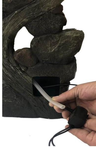
Attach the tubing to the pump. If needed, water flow can be adjusted using the flow control on the pump.
