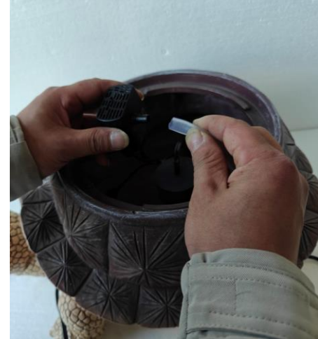
Attach the tubing to the fitting from the pump. If needed, water flow can be adjusted by the dial on the front of the pump.
