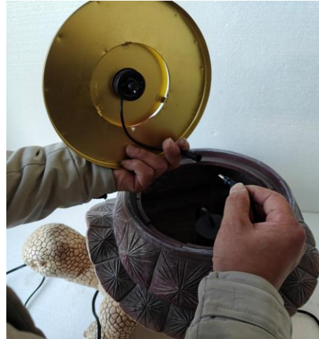
Locate the cable from the light and attach it to the corresponding connection from the pump.
