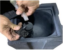
Locate the tubing and attach it to the pump.
