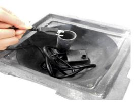
Pass the cord from the pump down the cord pipe and retrieve it at the base.
