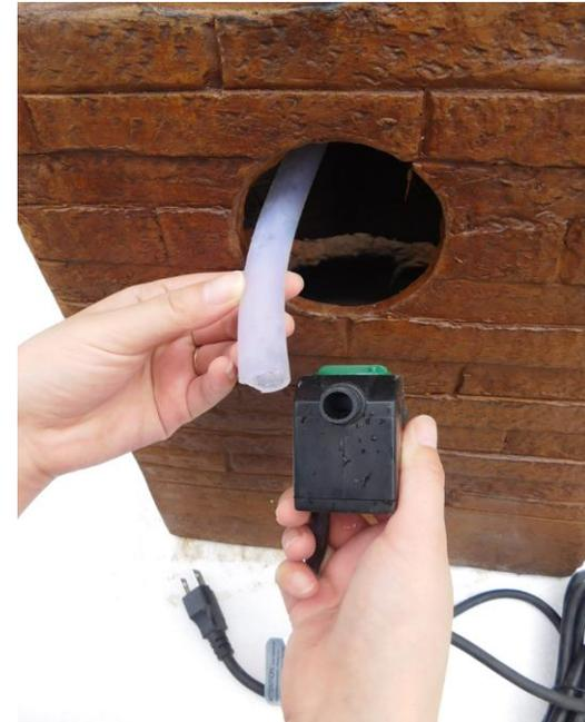
Locate the tubing and attach it to the pump. **Note:** water flow can be adjusted using the dial on the front of the pump. Place the pump inside the fountain.
