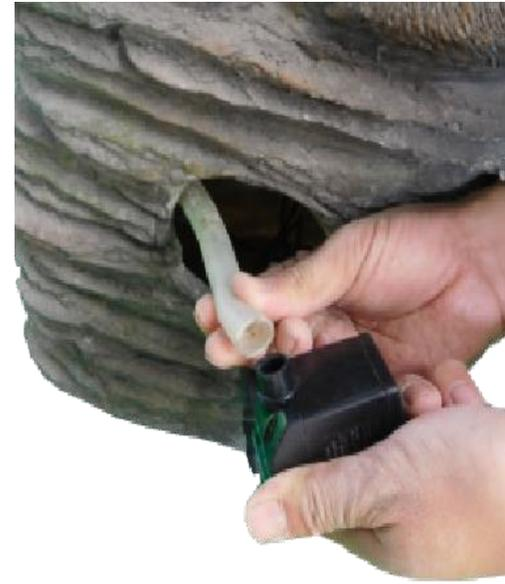
Attach the tubing to the pump. Water flow can be adjusted using the control on the front of the pump.
