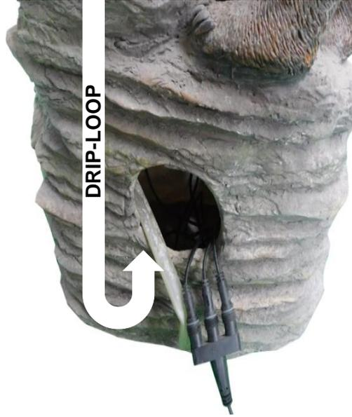
Retrieve the tubing and light connection. **The light connection must sit outside the fountain.** **IMPORTANT:** to prevent water loss during operation, create a drip-loop with the light cables by dipping them into the reservoir before they the fountain.
