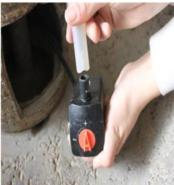
Connect the tubing to the pump then place the pump inside the housing. Install the pump access door.
