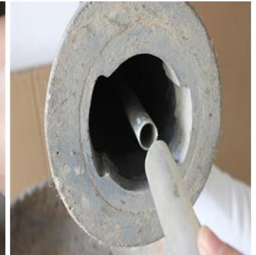
Connect the tubing to the top then pass it down the centre of the small bowl. Align, lower and lock the the top in place.
