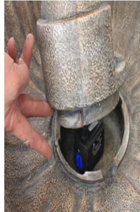
Set the pump housing / riser in to place, align the grooves then twist and lock it to the bowl.
