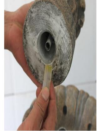
Connect the tubing to the top then pass it down the centre of the small bowl. Lower the top in place.
