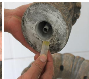
Connect the tubing to the top then pass it down the centre of the small bowl. Lower the top in place.
