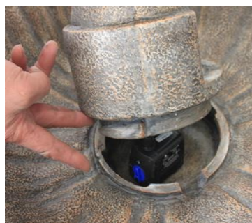
Set the riser in to place, align the grooves then lower and lock it to the bowl.
