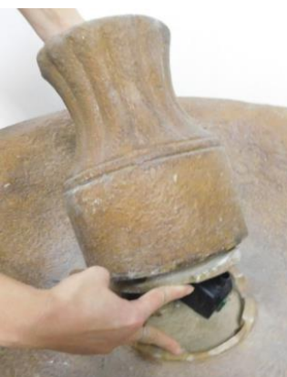
Align the pump housing and lower it in place. Twist and lock it to the large bowl.
