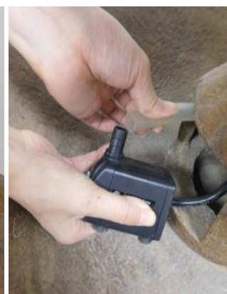
Locate the tubing from inside the pump housing and attach it to the pump.
