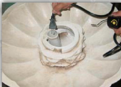
cord through standpipe
