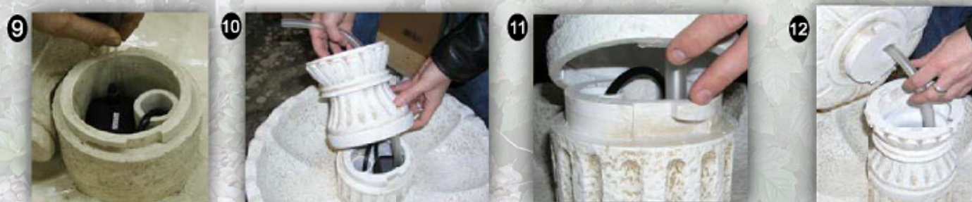
9. Attach tubing to pump 10. Pass tube through riser 11. twist and lock in place 12. tubing through bowl
