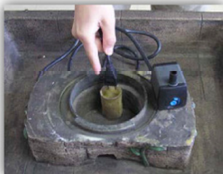
pump cord through standpipe in bowl
