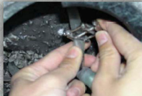
note location of restrictor to adjust flow. This unit is preset, but you may want to adjust top or bottom feature flow to achieve desired affect.
