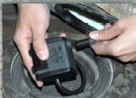
attach tubing connection to pump
