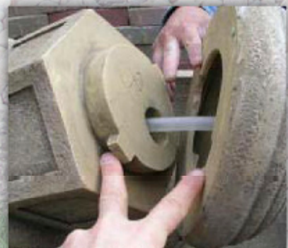
connect top to riser, can run overflow into riser if desired
