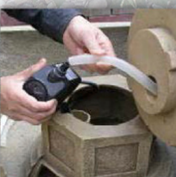
connect pump to tubing
