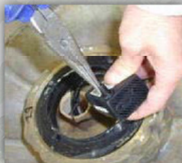
pull pump outlet out with pliers
