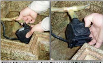
Attach tubing to pump. Note the position of the flow control, as it should be set to maximum as shown.
