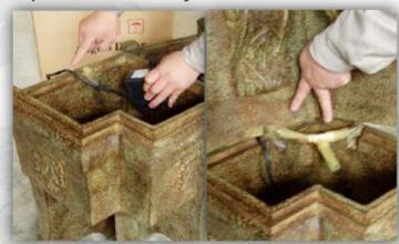
Place pump into far left groove, and put top in place so clear tubing fits into grooves without pinching.
