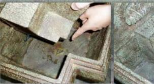
Pump cover is placed into bowl noting groove at bottom. It should sit level. Water level should remain higher than the "second step" to reduce splash.
