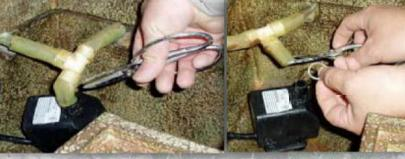
The most common problem is "kinked" tubing that will prevent proper flow and operation. You may have to trim the tube slightly for better fit. Check that the "T" connection fits securely over the tubing leading to the top, and all tubing is free from bending.
