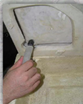
Insert tubing into nipple on top bowl, and fit into place.
