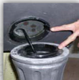
line up twist and lock (bowl to base)
