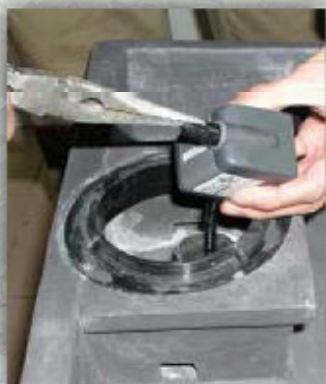
pull pump outlet out with pliers
