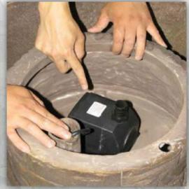
Run pump cord through pipe in housing. Pull through bowl, out bottom through groove. Pull out slack so pump sits as shown.
