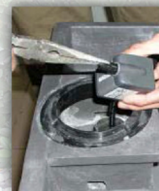
pull pump outlet out with pliers
