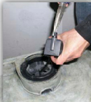
pull pump outlet out with pliers
