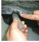
Align the tubing with groove at the base if kinking is a concern.
