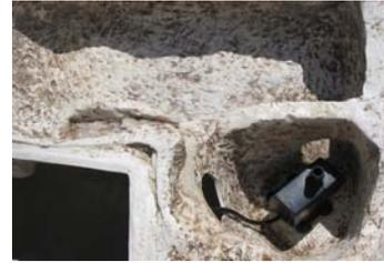
Place Pump in housing as shown. Run chord through pre-drilled hole and down the chord pipe provided.
