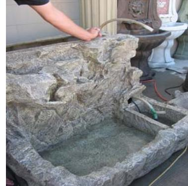
Pump should be placed in right section of bowl below section number 2. Use "T" connection to connect tubing already attached to section 2. Run long piece of tubing (supplied) up through body of section 1 through the access hole located near the pump. This will be your feed from the pump for the upper sections.
