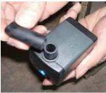
Insert black tube over pump output.
