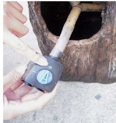
The pump is preset to full strength. If splash is a concern, reduce the flow as needed.
