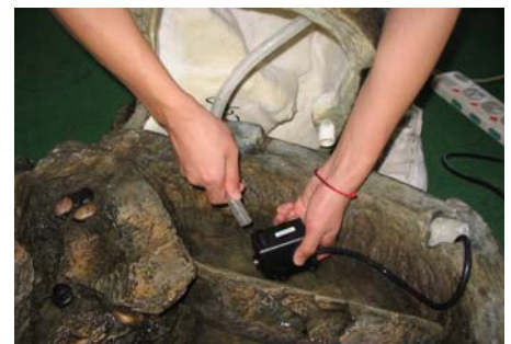
Connect the pump to the tubing from the top section of the fountain.
