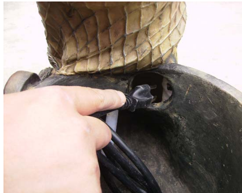
Pass the pump cord through the cord hole.
