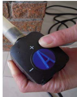
The pump is preset to full strength. If splash is a concern, adjust as needed.
