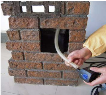
Locate the tubing from inside the reservoir and connect it to the pump.
