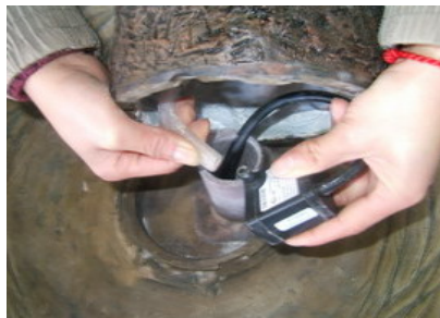
Connect the tubing to the pump, be sure it sits flat inside the housing without any kink in the hose.
