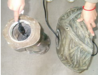
Pass the cord down the pedestal, and align with groove at the base.
