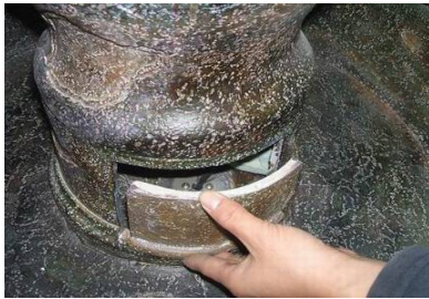
Install the pump access door.
