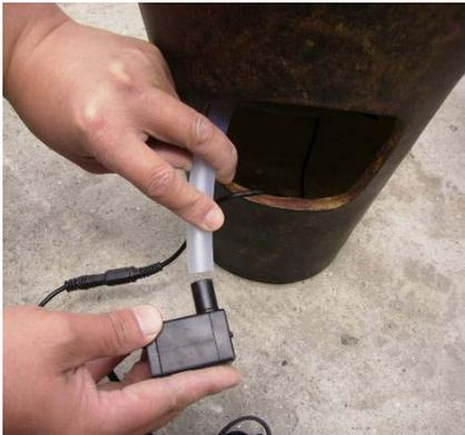
Attach the tubing to the pump.
