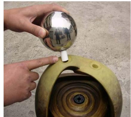
Install the larger orb by aligning the pin and setting in place.
