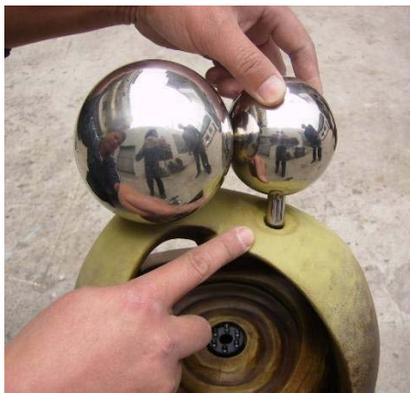
Install the smaller orb by aligning the pin and setting in place.
