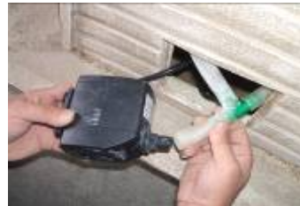
Connect the tubing to the "T", then connect the other end to the pump.
