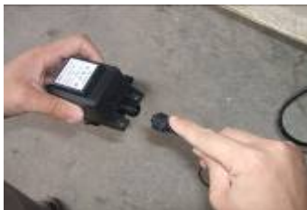
Connect the light cord to the transformer.
