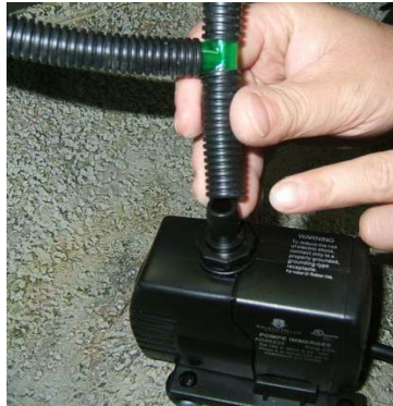
Connect tubing to the pump.
