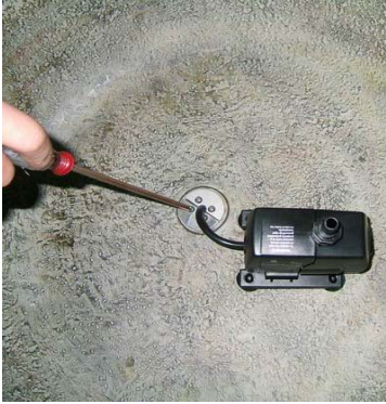
Pump comes pre-installed with cord seal. Check to see the cord seal is tight.
