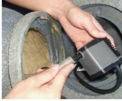
Make sure both power cord go through pvc pipe, lead to the groove at bottom. Insert rubber bung as shown.
