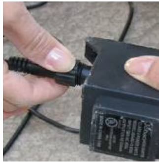
Make sure both power cord go through pvc pipe, lead to the groove at bottom. Insert rubber bung as shown.
