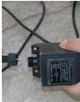
Make sure both power cord go through pvc pipe, lead to the groove at bottom. Insert rubber bung as shown.
