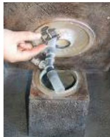
Connect tubing to upper bowl and adjust restrictor to desired setting. Twist and lock upper bowl into place.
