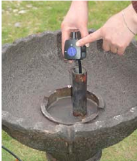
The pump is preset to full strength. If splash is a concern, adjust as needed.
