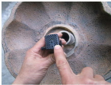
Pump is preset to full, adjust lower if less splash is desired. Be sure it sits flat inside the housing without any kink in the hose.
