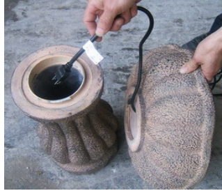
Insert cord through pedestal. Align with groove in the base.
