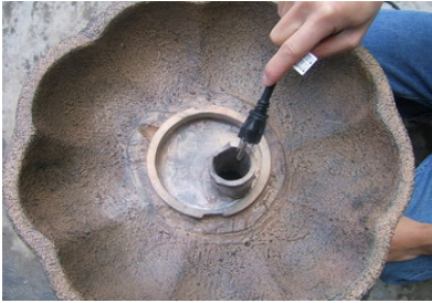
Pump cord through cord pipe.
