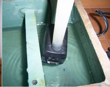
To connect the pump, set the main body at an angle on the base as shown, and connect the tubing to the pump. Set the pump to the desired setting. Place the main body on to the base.
