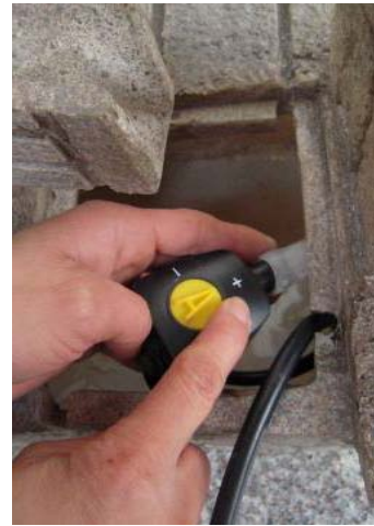
The pump is preset to full strength. If splash is a concern, adjust as needed.
