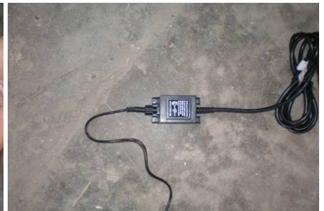
Attach light cord to transformer. Be sure it is tight. Place transformer in a secure area, preferably under cover. While this unit is rated for outdoor use, it should not be fully submersed in the water.
