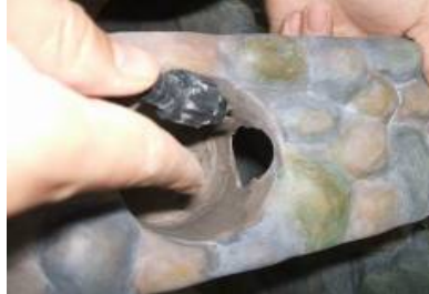
Run the light cord through the cover plate, then through PVC pipe.
