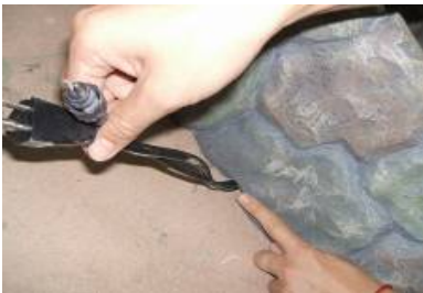
Make sure both power cord go through pvc pipe, and align with the groove at the base.
