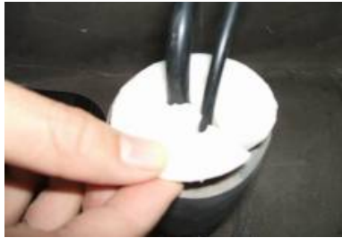
Run the light cord through the cover plate, then through PVC pipe.
