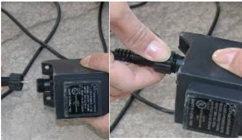
Attach light cord to transformer. Be sure it is tight as shown. Place transformer in secure area, preferably under cover. While this unit is rated for outdoor use, it should not be fully submersed in the water.
