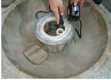
Feed the pump cord through the cord pipe.
