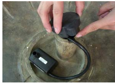
Place the cord pipe cover over the cord pipe as shown above.
