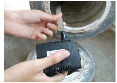
Connect the tubing to the pump.
