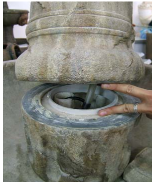
Twist and lock the top to the pump housing.
