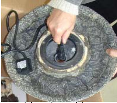
cord through standpipe
