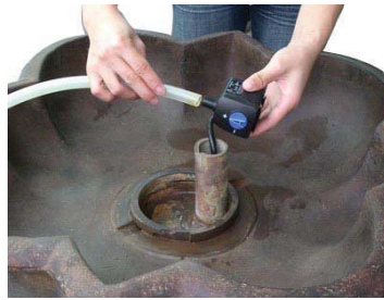
Connect the tubing to pump.
