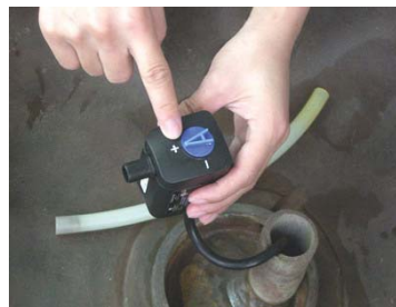
The pump is preset to full strength. If splash is a concern, adjust as needed.
