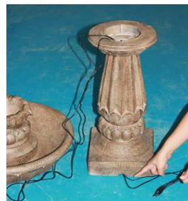
Align the cords from the pump and light with the groove at the base of the pedestal.
