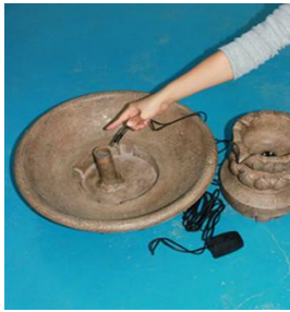
Pass the light and pump cords down the cord pipe in the bowl.
