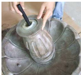
"Twist and lock" riser in place.
